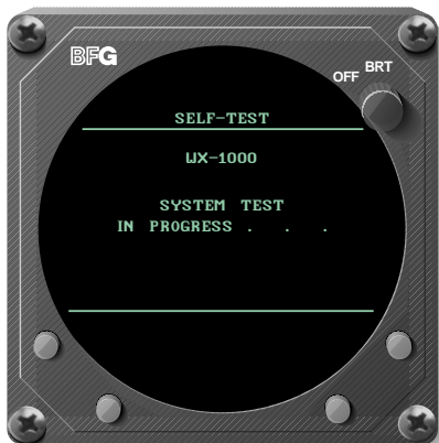
Figure 3-2. System Test in Progress
